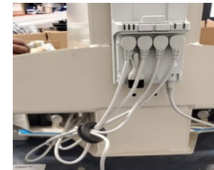
Re-routed cables with adaptors installed
