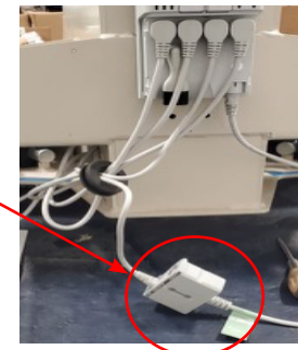
Re-routed cables with adaptors installed
