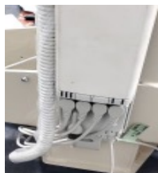
Attached cover and junction box
