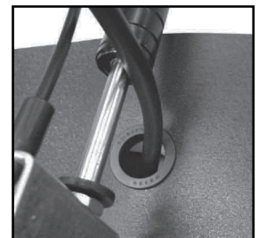
Insert Cable Connector Labeled SEAT Through Bushing
