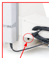
Rubber O-Ring Route Cable Here
