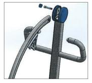
4. Attach boom to top of mast and place the blue plastic soft cover on top of mast and boom as shown above.
