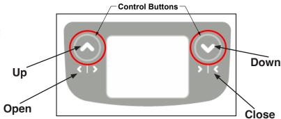
Mast appears in orange color. Press "up/open" button, for lift to go up.
