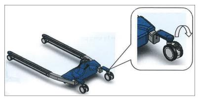
1. Engage the lift brakes as shown above.
