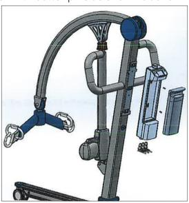
6. Attach the control box bracket to the mast with the two screws, then attach the control box to the mast with the two screws, then slide the battery in until it snaps into place, as shown above.
