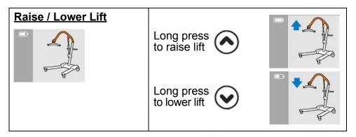
1. Press the button to raise or the button to lower the lift.
