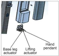
7. Insert the actuator and hand pendant connectors as shown above.
