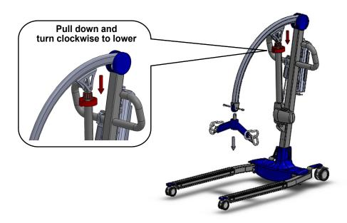
The device consists of a plastic collar ring that should be pulled down, then turned clockwise continually until the patient has been lowered.
