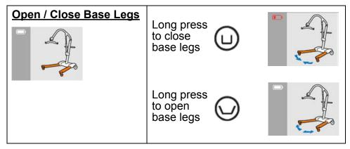
2. Press the O button to open or the O button to close the lift base legs.
