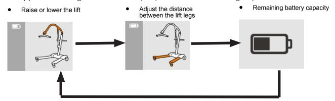
Legs appear in orange color. Press "up/open" button, for power base to open.
