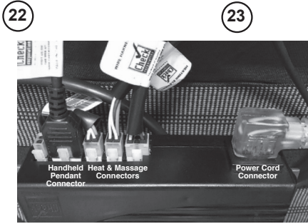
24 Heat and Massage Feature – Control Module and Transformer Unit Showing All Connections Correctly Made
