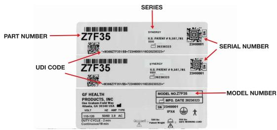
Bed labels are an important part of identifying the bed's make and model when ordering replacement parts. The Serial Number is essential if you are claiming parts or service under warranty. These helpful labels can be located on the main frame rails, immediately below the sleep decks on either side of the bed.
