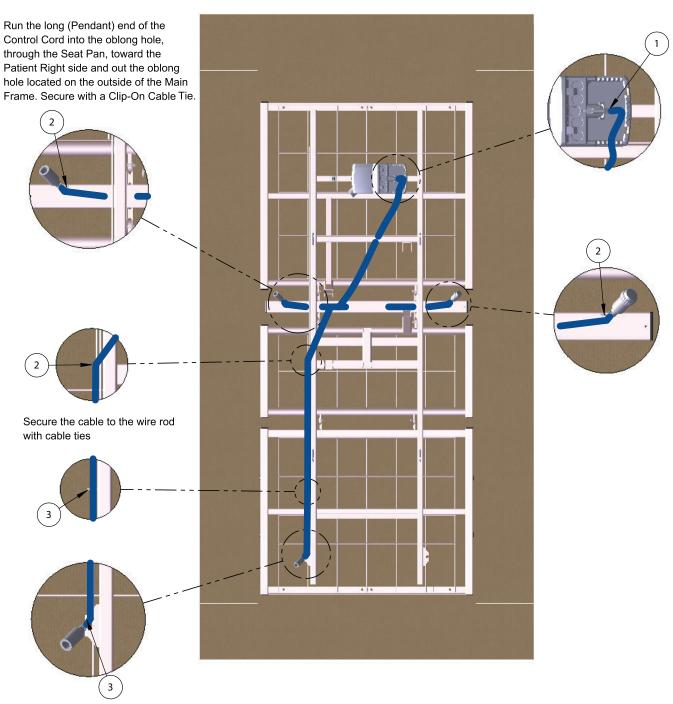
Run the longest (Staff Control) end of the Control Cord along the Main Frame Rail toward the Foot-End of the bed.
