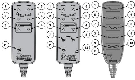
ZENITH SERIES WITH STANDARD POSITIONING HAND CONTROL PENDANT ZENITH SERIES WITH ADVANCED POSITIONING HAND CONTROL PENDANT OPTIONAL ACCESSORY: ZENITH SERIES WITH TRENDELENBURG / REVERSE TRENDELENBURG HAND CONTROL PENDANT
