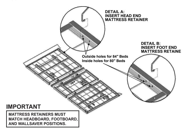
Be sure to use a mattress that is properly sized to fit the sleep deck, which will remain centered on the deck relative to State and Federal Guidelines. Use of an improperly fitted mattress could result in injury or death.
