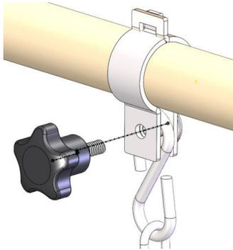
6. Holding the bracket in place, insert the handle through the male bracket piece and screw into the weld nut connected to female bracket (as shown).
