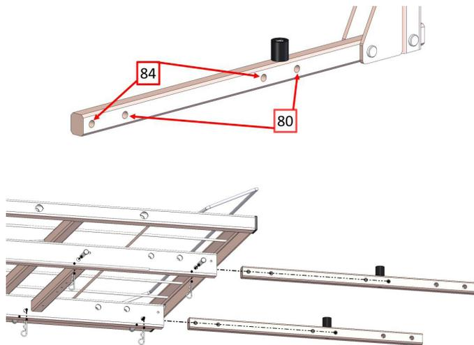
3. Assemble trapeze adaptor weldment to the mounting bar, then mount headboard to the trapeze adaptor.
