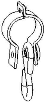
5. Place bracket around the top of the trapeze bar (as shown).
