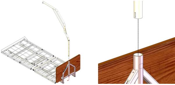
3. Insert the male bracket tab through the female bracket's hole.
