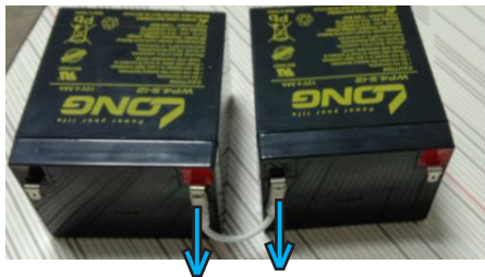
Unplug Terminal from Old Batteries (Pull Up)
