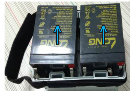
Remove Both Batteries by Pulling Up Both Batteries at the Same Time
