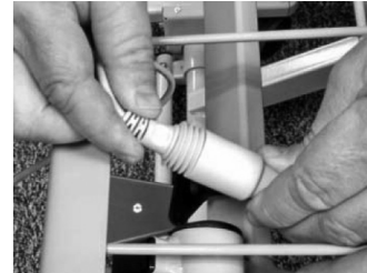
Proper Connection (completely seated)
