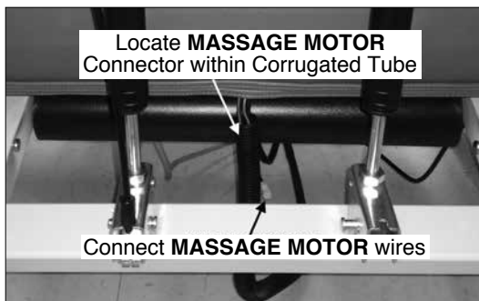
Connect Massage Motor Wires
