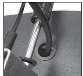
Insert Cable Connector Labeled SEAT Through Bushing
