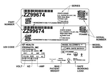
Bed labels are an important part of identifying the bed's make and model when ordering replacement parts. The Serial Number is essential if you are claiming parts or service under warranty. These helpful labels can be located on the main frame rails, immediately below the sleep decks on either side of the bed.
