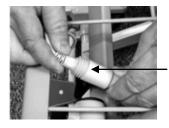
Proper Connection (completely seated)
