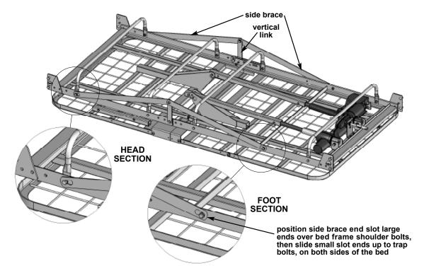
4. Position the truss assemblies on both sides of the bed so that the vertical truss links face the middle of the bed and the side braces are on the outside. Position the side brace end slot large ends over the protruding welded shoulder bolts near the ends of both the head and foot section frames, then slide the small slot ends over the shoulder bolts so that the bolts are trapped in the small slot ends, as shown above.
