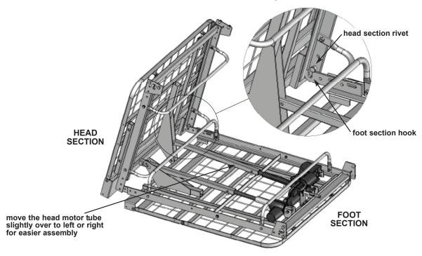
2. Move the head motor tube slightly over to the right or left to get it out of the way. Using two people, lift the head section so that it stands perpendicular to the foot section as shown above. Lift the head section and align the two rivets (on either side of the inside frame) with the two hooks in the foot section frame, as shown above. Lower and slowly maneuver the head deck so that the rivets seat in the hooks.
