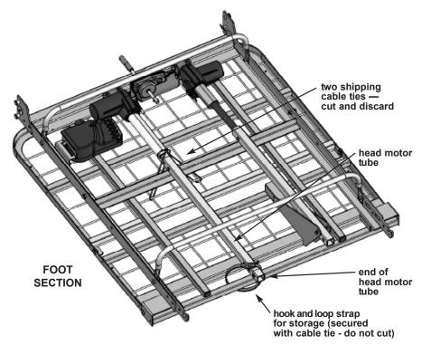
REMOVE SHIPPING CABLE TIES FROM HEAD SECTION TRUSSES
