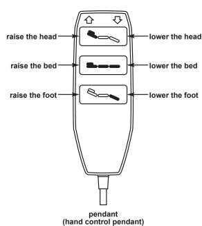
If any of the pendant functions do not work as expected, recheck all electrical connections to ensure all cables are seated properly within the motors and the control box, then retry the pendant function that did not work.
