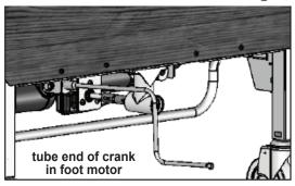
To lower the bed platform with the emergency crank, insert the crank's flat end into the HI / LO motor shaft slot as shown at above left and turn it counterclockwise.
