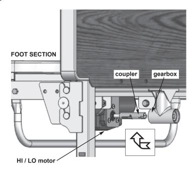
4. Once the coupler is unlocked, the inner spring will force it toward the foot end gearbox located at the bottom of the bed end assembly. The HI / LO motor shaft cross pin should now rest at the end of the long groove in the coupler, and the end of the coupler should rest inside the gearbox and engage the gear shaft.
