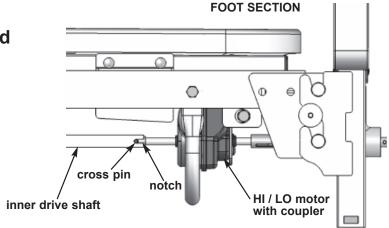
6. At the head end, depress the small spring-loaded inner drive shaft, and place the shaft end notch on the head end gearbox shaft cross pin as shown at right.
