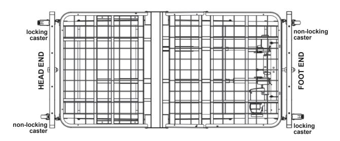
Info: Before installing the two locking and non-locking casters, ensure they will be easily accessible once the bed ends are attached. For best results, position the two locking casters so that they are diagonally on opposite sides of the bed as shown above.
