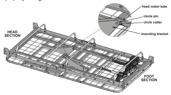
3. Carefully lower the head section to the floor, ensuring the head section rivets remain engaged in the foot section hooks. Remove the clevis pin and circle cotter, shown above, from the head section's mounting brackets. Lift up the head motor tube and place it so that it rests between the two brackets and the first hole lines up with the bracket holes. Insert the clevis pin and secure with the circle cotter, as shown above.
