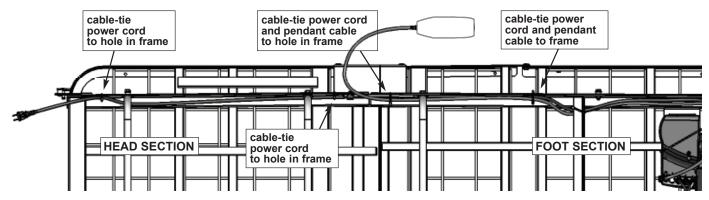
The head section of the bed does not come with any cable routing. The power cord and pendant cables will be coiled and cable-tied to the foot section in packaging. To route the power cord and pendant cable:
