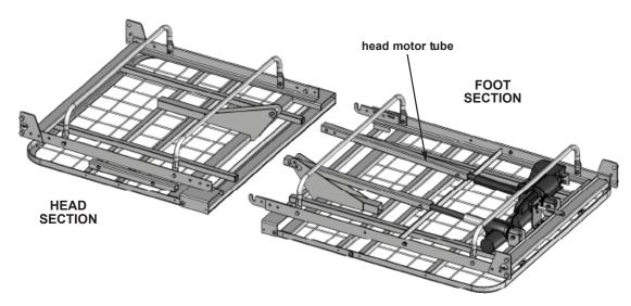
1. Lay the bed's foot section (with motors and junction box) upside down, flat on the floor, as shown above. Do the same with the head section close by.
