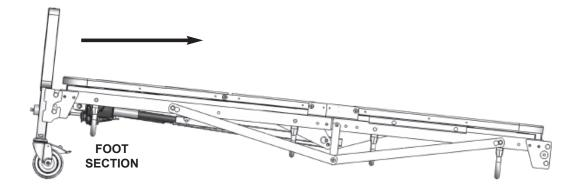
3. Once the rivets are aligned with the hooks, tilt the bed end forward, toward the foot section as shown above, then lower the bed into the hooks to lock into place. Do the same for the head end of the bed, repeating steps 2 and 3.
