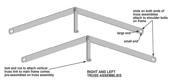
The two truss assemblies, shown above, span the decks and give them more stability, much like the trusses on a bridge. The trusses attach to the main frame via welded shoulder bolts on either side of the head and foot sections.
