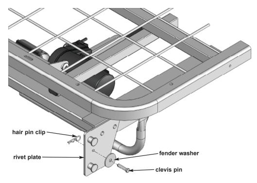
1. You must first remove the bed end locking hardware (clevis pins, washers, and hair pin clips, total 4 each) from the frame rivet plates on both sides of the bed before you can attach the bed ends. The bed end locking hardware has been pre-installed at the factory for ease of shipment, and will be reinstalled after installing the bed ends to act as latches when the bed ends are attached to head and foot sections.
