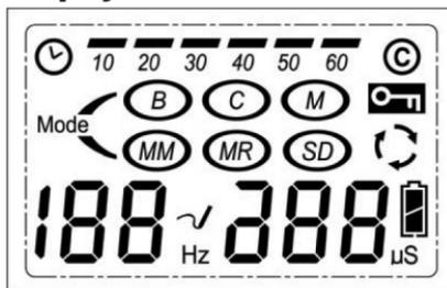
The LCD displays timer (10, 20, 30, 40, 50, 60 minutes and © continuous), function modes (B, C, M, MM, MR, SD), alternate mode, pulse width, pulse rate, low battery, and patient compliance counter.
