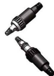
DETAIL B: ENSURE LOCK END CAPS ARE SCREWED ON SECURELY
