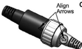
DETAIL B: ENSURE LOCK END CAPS ARE SCREWED ON SECURELY
